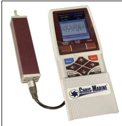
Fig.1.: Mitutoyo Surftest SJ-210 surface roughness tester
